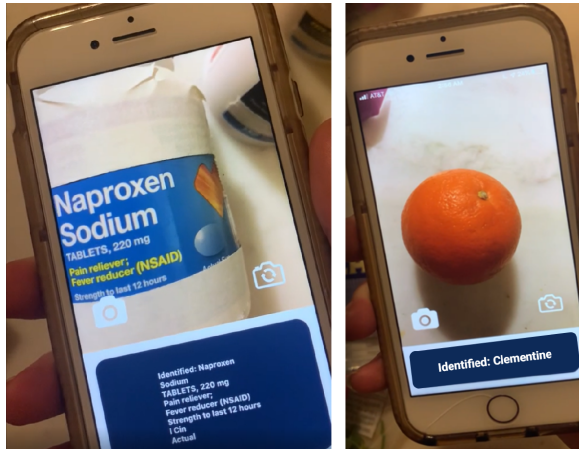
Figure 3. Identification of medicine bottle labels (left) and grocery items (right). Note that the text labelled on the bottom is for supplementary purposes to confirm accuracy of identification, as the text would not be easily visible for visually impaired users.
